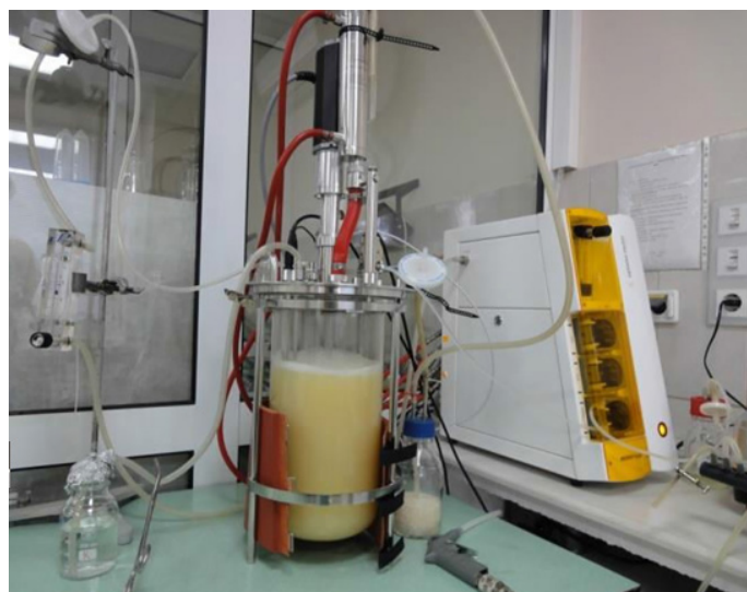
Figure 11: Cultivation process by C. laurentii AL 65 in a Bioreactor Sartorius Biostat Aplus.
